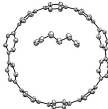
Figure 2. ORTEP drawing of [10]CPP·hexane. Thermal ellipsoids are shown at 50% probability, and all hydrogen atoms are omitted for clarity.
